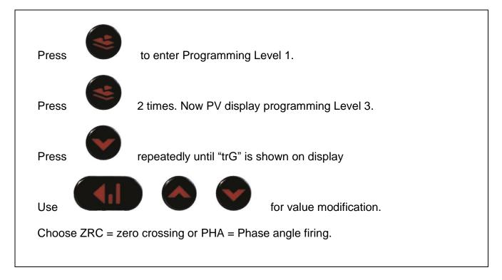
Phase angle firing is preset from factory on the MTX-51.
