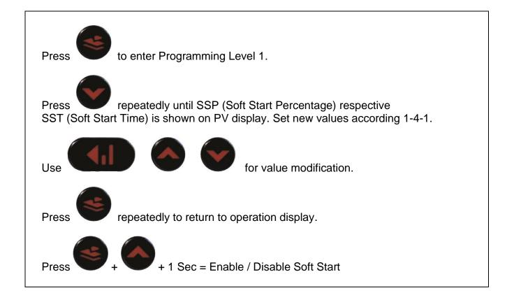
SST (Soft Start Time) = 0 minutes means the soft start function is disabled. **Not recommended**.
